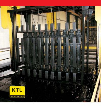
Our lifting mechanisms are also protected with KTL layer as standard. This minimises the consequences of stone chip damage and prevents spreading rust. The KTL coating has been subjected to a Salt-spray test:
