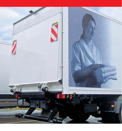
Special applications require special equipment. With its exceptionally large load clearance of 1000 mm and its lifting capacity of 2500 kg, the 2500 KK is rightly considered one of the most powerful tail lifts in its class. It is designed for a wide range of applications such as food and beverage distribution, and for drawbar units.
