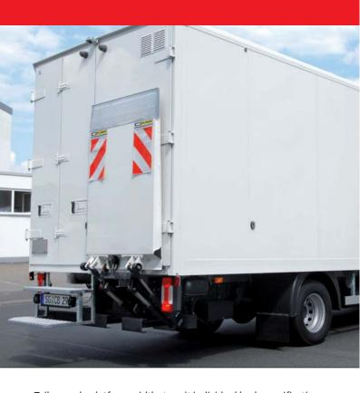
Tailor-made platform widths to suit individual body specifications, where access to the rear of the vehicle is required without lowering the tail lift platform. Particularly ideal for refigerated vehicles allowing clear entry through one door which may be fitted centrally or to the near or offside.
