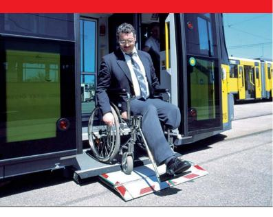
The MEDILIFT range of fully automatic, electrically operated lifts is designed for low-floor trams and buses, providing safe and easy access for wheelchair users. The MEDILIFT is particular useful in areas with no pavements as all passengers, not only wheelchair users, can enter the vehicle with ease.
