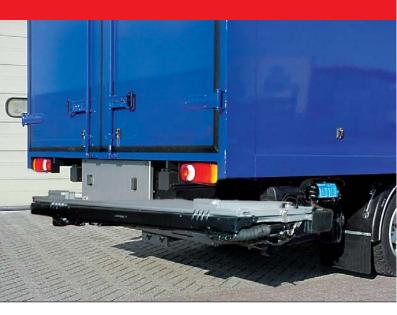
Robust retractable lift available in two capacities with double folding platform ideal for vehicles with short overhangs (from 985 mm). Stowing 'completely' out of the way under the rear of the vehicle it is ideal for fork lift and dock loading operations. Suitable for dry freight and refrigerated applications.
