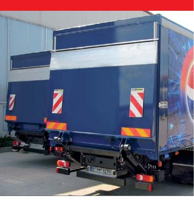
A versatile standard cantilever featuring a lightweight aluminium platform lifting 1500 kg. Designed to maximise vehicle payload, it is available in a wide range of platform sizes to suit many applications. The 4-cylinder lift mechanism provides optimal performance. Suitable for floor heights up to 1546 mm.
