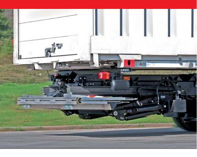
The 2000 KLUZ is a robust lightweight retractable lift. A push-pull cylinder aligned lengthwise moves the lift into the desired position. The lift leaves the factory fully assembled and with the lift unit KTL coated, ready for clamping onto the chassis supplied with kits suitable for trucks or trailers.
