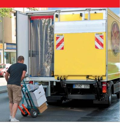
These tail lifts are based on the well-proven K series. They offer a wide range of applications and are tailored to the transportation of fresh or chilled goods. The rear of the truck may be accessed without lowering the 1/3 or 2/3 width platform which may be mounted to the left (K1TL) or right (K1TR) side of the vehicle. Platform widths from 800 mm to 1960 mm.
