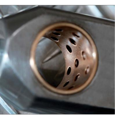
A series of lubrication holes evenly distributed guarantee an equal application of grease.
