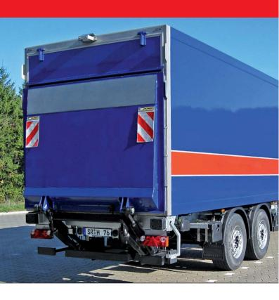
The 2500 KL is the No. 1 Tail Lift for all heavy goods applications. Lifting a full 2500 kg at a load distance of 750 mm it is available with both aluminium and steel platforms. A wide range of options, including a choice of 4 different lift arms, makes it suitable for virtually all heavy load transportation requirements.
