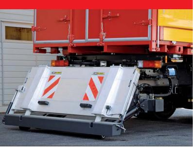
Robust retractable lift with double folded platform ideal for vehicles with demountable bodies and also fixed bodies with short overhangs. The lift including the retraction unit leaves the factory fully assembled with the lift unit powder coated. When stowed, the lift forms the vehicle's underrun bumper. The lift is entirely operated by a user friendly K-plus control system and optional EasyMove control. Ideal for frequent use.
