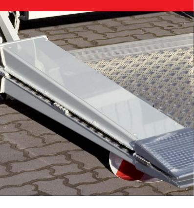
AluStar is the most versatile aluminium platform on the market. Since it is not of modular build we can meet customer requirements by cutting the platform to the required width and depth to suit individual applications. Side ramps can also be added if required.
