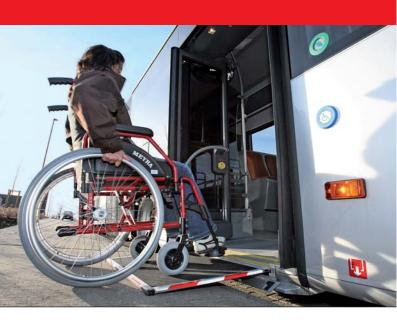
The range of MEDIRAMPE ramps includes both fully automatic and manually operated models designed for use in low-floor trams and buses providing easy and safe access for wheelchair users.
