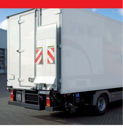
These tail lifts, based on the well-proven AQ series, are suitable for a wide range of applications and are especially suited for fresh or chilled goods. The platform (available 1/3 or 2/3 widths) need not be lowered to access the rear door and may be mounted to the left (AQ1TL) or right (AQ1TR) side of the vehicle. Platform widths from 800 mm to 1960 mm.
