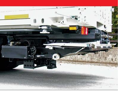
Robust retractable lift available in two capacities specially designed for drawbar applications. Stowing 'completely' out of the way under the rear of the vehicle it is ideal for fork lift and dock loading operations. Suitable for dry freight and refrigerated applications.
