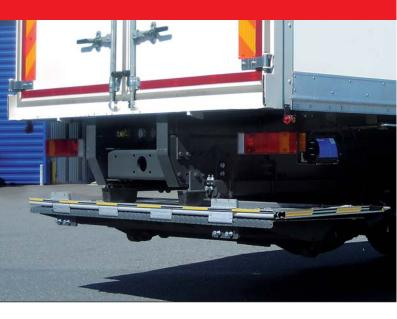
A specially designed retractable tail lift for easy assembly on vehicles with a frame width of approximately 750 - 865 mm. The guide rails are included in a frame and can be assembled without requiring adjustment.
