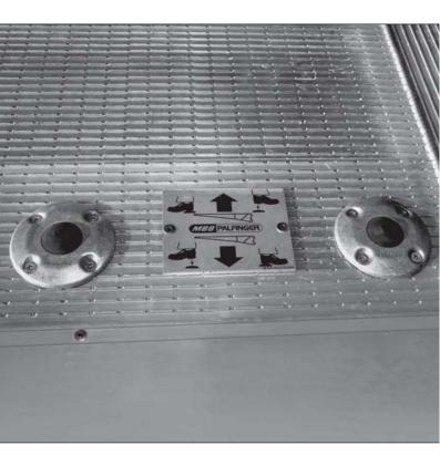
Our 'Intelligent' foot controls are able to distinguish between contact with the operator's foot and the load! Should goods be resting on the foot controls the lift remains static.
