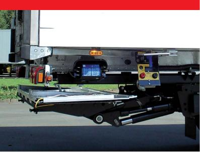
A specially designed retractable tail lift for easy assembly on semitrailers with a frame width of approximately 1300 mm.
