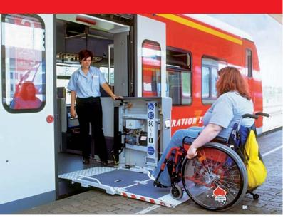
The range of semi-automatic TRAINLIFT-products provides safe and easy access for wheelchair users travelling by rail. Stowed neatly inside the entrance to the carriage, the platform pivots round and lowers, bridging the gap between the carriage floor and the platform. For reasons of safety the lift is stowed locked and can only be operated by authorised personnel. The TRAINLIFT is designed for lifting up to 1200 mm.
