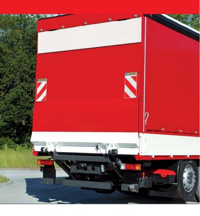
2000 KL is a powerful tail lift for demanding applications that require a lifting capacity of 2000 kg with a load clearance of 750 mm. 5 different lift arms and models with aluminium or steel platforms are available. A wide range of options are available, to meet the requirements of virtually all applications.
