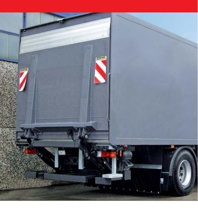
Lifting a full 2000 kg, the 2000 K offers a choice of steel or aluminium platforms, up to a maximum depth of 2800 mm and is frequently chosen for use by the food and drink distribution industry. The 4-cylinder lift mechanism is available with four different lift arms, ranging from 700 mm to 1100 mm.
