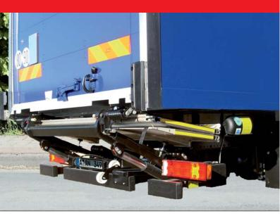
The TwinFold is a light weight, 2-cylinder tuckunder lift with a lifting capacity of 1500 kg. Its folding platform stows under the vehicle chassis, providing clear access to the rear of the vehicle when required. Platforms available 1200 mm and 1400 mm deep. Designed for dry freight applications, it is ideal for the lifting of pallets and roll cages. With its two lift cylinders and two parallel struts, the TwinFold lift offers full stability. Mechanical auto-tilt at ground level.
