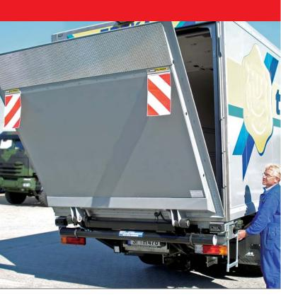
This special lift is designed for fitting to vehicles with a deep coupling system. It uses well-proven standard components of 1500 K and 2000 K lifts. The single-piece underrun bumper is spring-loaded and, on request, hydraulically pivoting. The long lift arm (1100 mm) permits level mounting of the platform.
