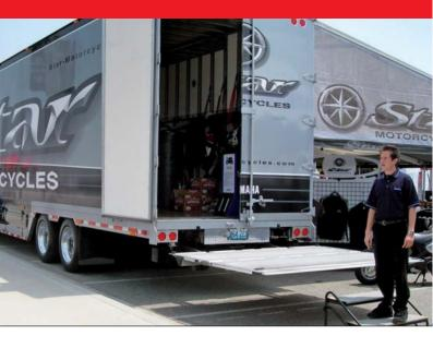
This heavy duty retractable lift is available in two capacities. Stowing 'completely' out of the way under the rear of the vehicle it is ideal for fork lift and dock loading operations. Suitable for dry freight and refrigerated applications.
