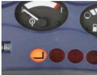
Lifting interlock lamp on the control panel
